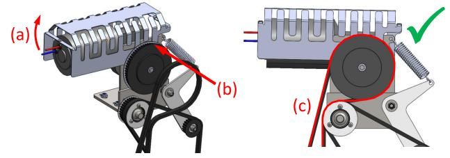
STEP 7: Realign position of motor (a) with marking and re-tighten (3) motor fixture screws (b).
