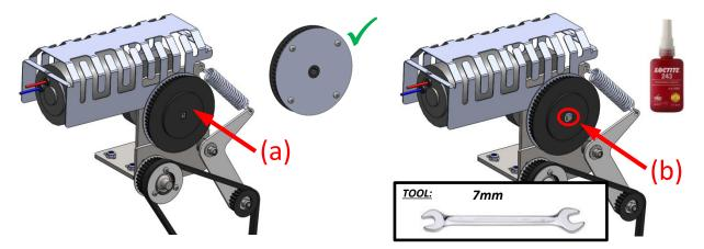
**STEP 6:** Lift motor (a) and reinstall belt on new pulley (b). Take care about correct belt routing (c).
