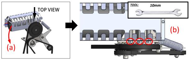
STEP 8: To ensure proper belt tension, you should be able to twist belt 360 degrees (+/-30 degrees).
