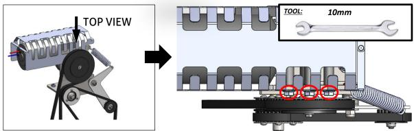
STEP 3: Lift motor (a) to relax belt then remove belt (b) from pullev.
